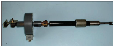
Fig.6.1. The inductive force transducer with the didactical magnetorheological damper.
