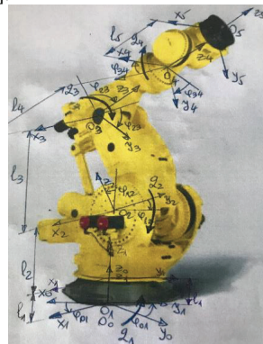
Fig.5.14. The arm type studied robot
