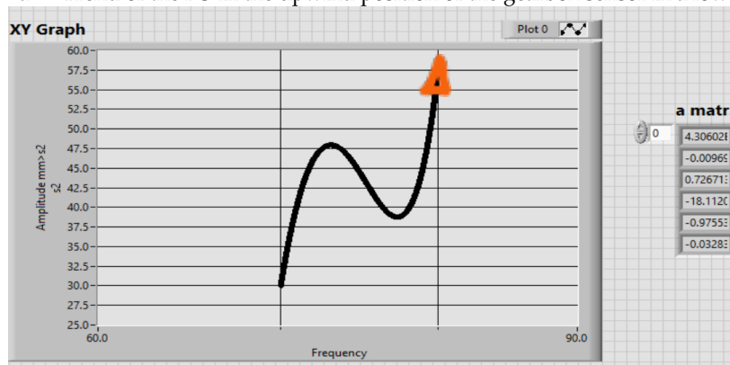
b- Trend of the FO in the upwind position of the gearbox sensor in a high frequency.
